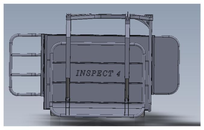
Overall length of crate in down position from end of frame at back to squeeze door: 3.25meters
